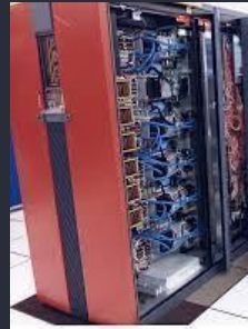
Cray YMP Cold Plate Pumped Fluorinert Cooled
